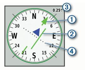
The course pointer ① indicates your relationship to the course line leading to the destination. The course deviation indicator (CDI) ② provides the indication of drift (right or left) from the course. The scale ③ refers to the distance between dots ④ on the course deviation indicator, which tell you how far off course you are.
