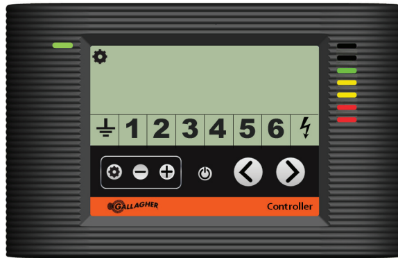
Controller showing the output voltage being adjusted
